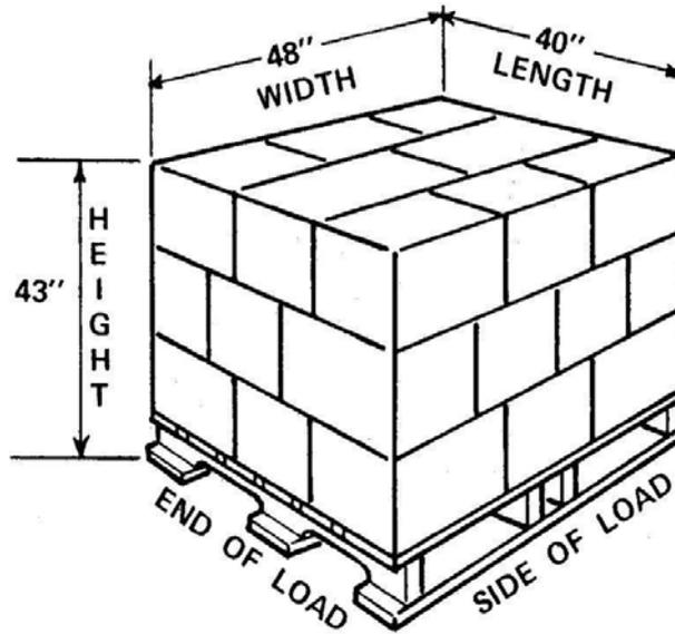
FIGURE 2. Palletized unit load sizes (see 5.1.1.1).
