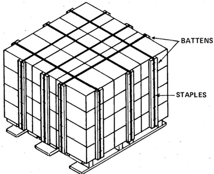
FIGURE 48. Stability dunnage type 20 (cross-strap battens) (see 5.4.11.1).
