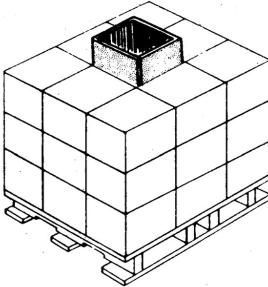
FIGURE 52. Stability dunnage type 28 (chimney filler) (see 5.4.16).
