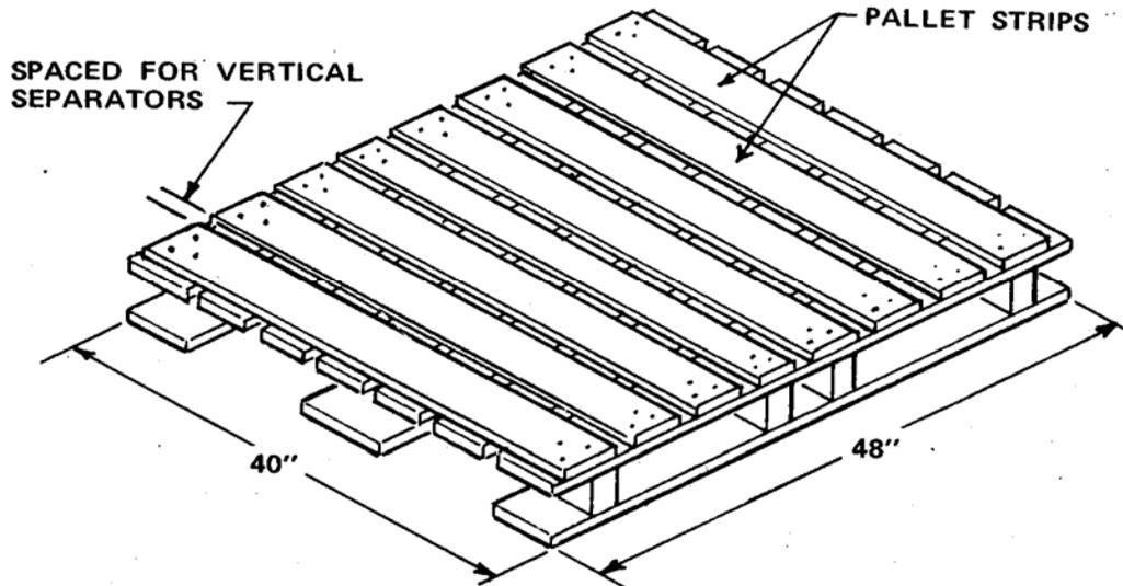
FIGURE 47. Stability dunnage type 19 (pallet strips) (see 5.4.10).
