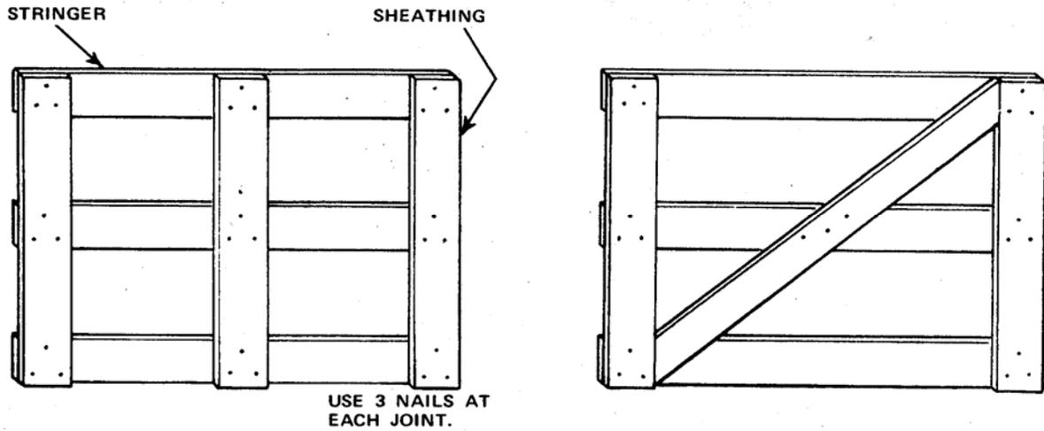
FIGURE 44. Top, side, or end frame (typical) (see 5.4.6).
