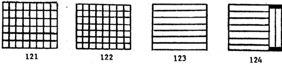
FIGURE B-1. Load patterns on 40- by 48-inch pallets (see A.2.2) (continued).
