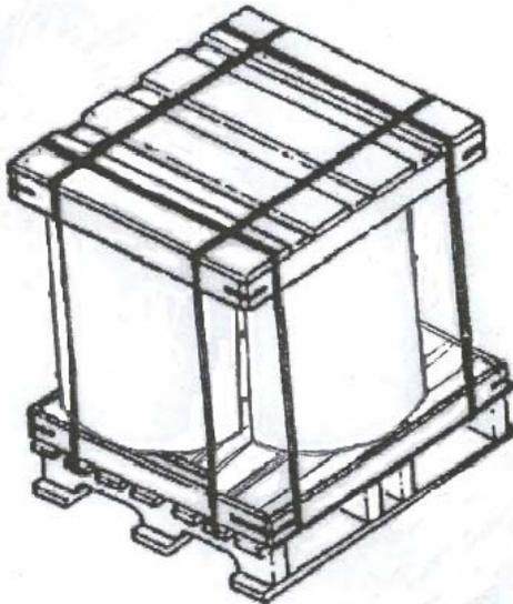
FIGURE 20. Load type XIIc (strapped) (see 5.2.12.3).
