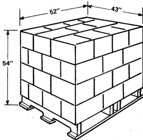
FIGURE 3. Other palletized unit load sizes (see 5.1.1.2).
