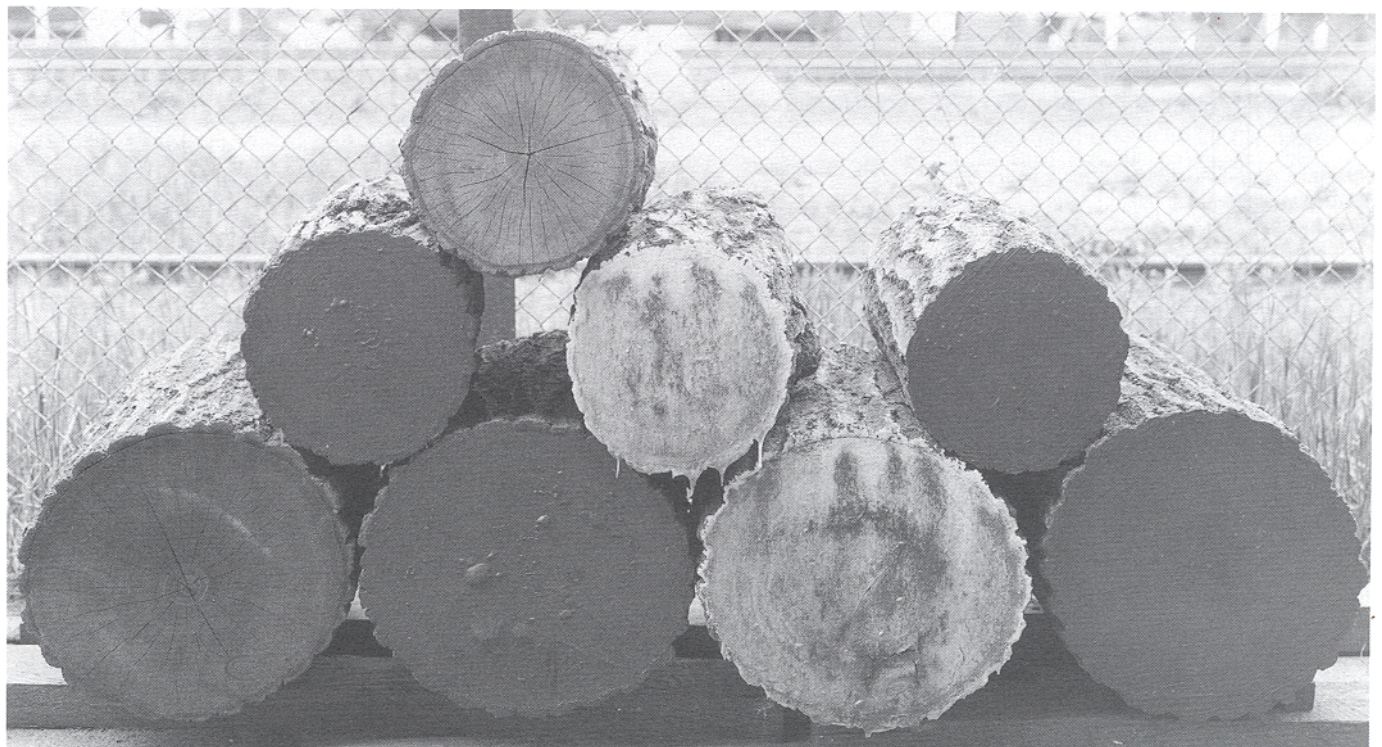
Figure 10-3—Oak logs 8 months after they were cut and the ends treated with preservatives. All but two logs were also end sealed; no end checking developed in these logs. The preservative treatment of the unsealed
