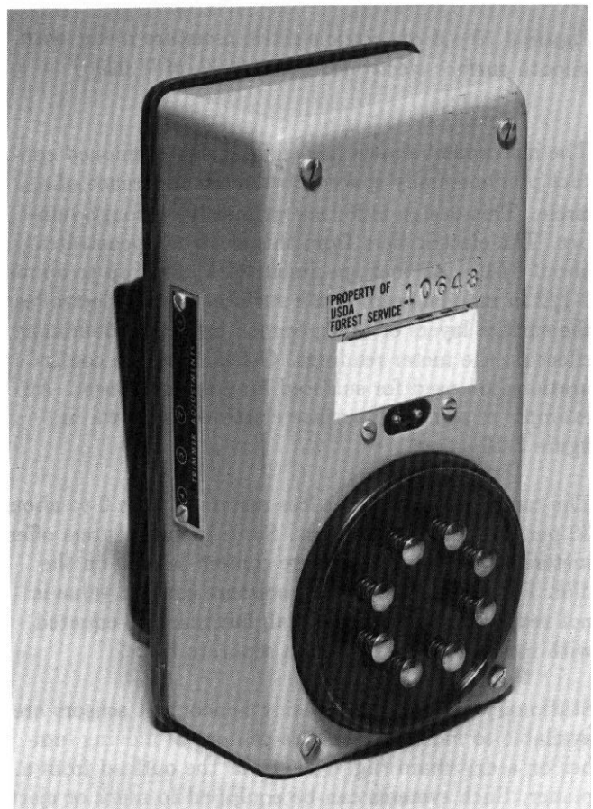
Figure 3-9 —A radiofrequency power loss type electric moisture meter. (M 133689)
