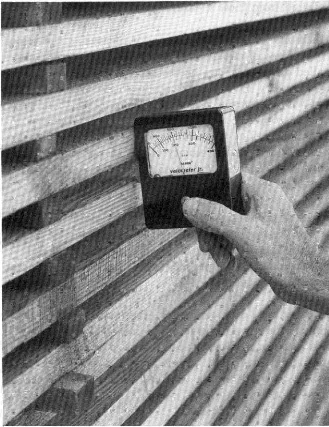
Figure 3-21 —Deflection anemometer. A type of air velocity meter. (M87 0194-13)
